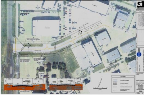
Above: Exhibit A from the Preliminary Engineering Report (PER) produced by Garver shows the extent of the Taxilane Victor reconstruction project. Two representative pavement cross-sections are shown at the bottom of the drawing. Preliminary calculations indicate that 12 inches of concrete over a compacted aggregate base will be required to support the large aircraft that are presently using this taxilane.
