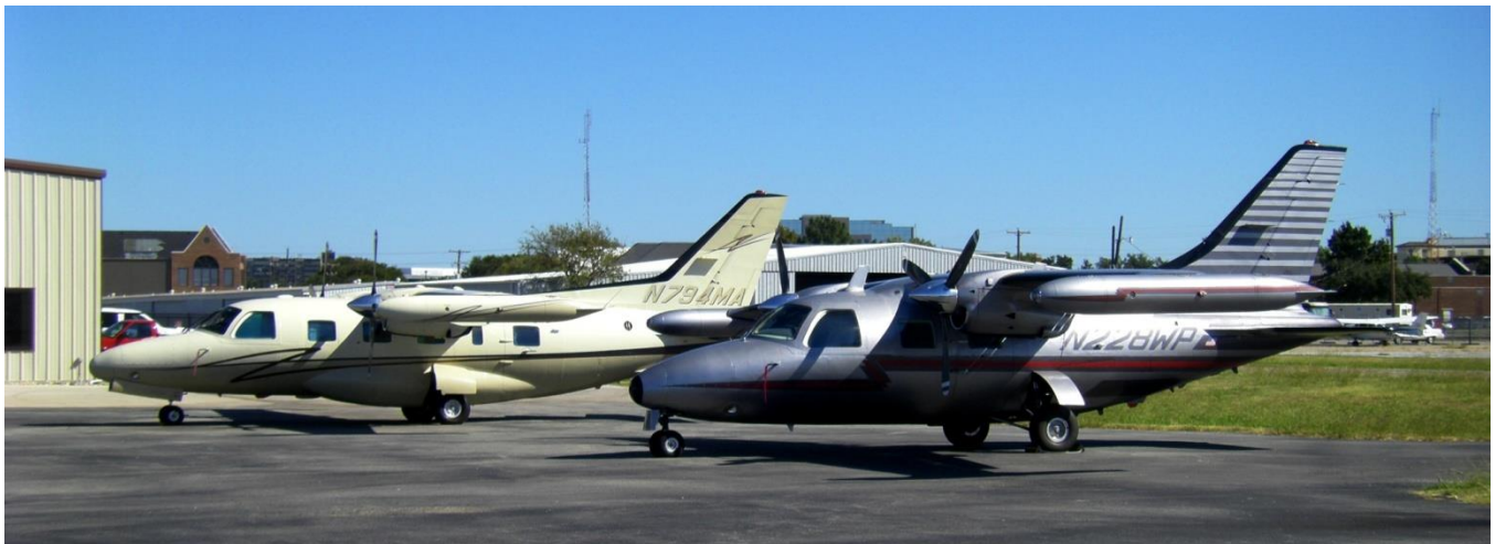
Above: A pair of Mitsubishi MU-2s on the ramp at Turbine Aircraft Services. At left is a long-fuselage variant MU-2B-60 “Marquise”, while at right is a slightly older MU-2B-20 short-fuselage variant. The short-fuselage variants are frequently referred to as “Solitaires” although strictly speaking only the MU-2B-40 was called the “Solitaire” by the manufacturer (and similarly for the long-fuselage variants, which are usually all called “Marquises”). Regardless of what version of MU-2 you may fly – and there are still around 230 MU-2s in the active U.S. fleet – Turbine Aircraft Services at Addison Airport is the place to go for MU-2 product support.
