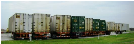
Below: 53-foot shipping containers filled with aerated concrete EMAS blocks are staged on the run-up pad at the south end of Taxiway Alpha.
