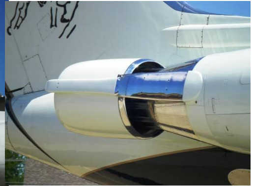
Above and Left: “Hushkits” fitted to the engines of these Gulfstream G-III aircraft reduce the noise emissions to Stage 3 levels, enabling the continued operation of these aircraft beyond December 31, 2015.
