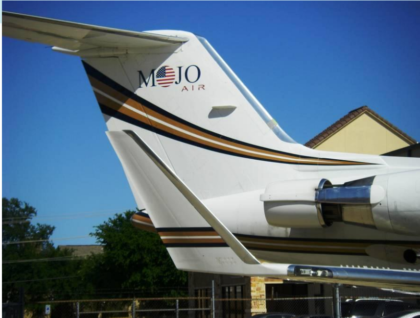
Above and Left: “Hushkits” fitted to the engines of these Gulfstream G-III aircraft reduce the noise emissions to Stage 3 levels, enabling the continued operation of these aircraft beyond December 31, 2015.
