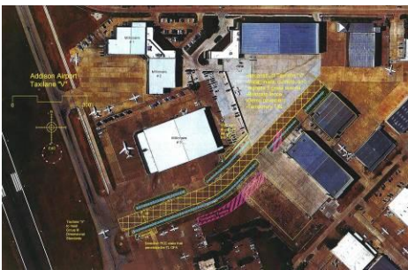
Above: an overview of the proposed work on Taxilane Victor, including pavement reconstruction, drainage improvements, and a temporary taxilane.
