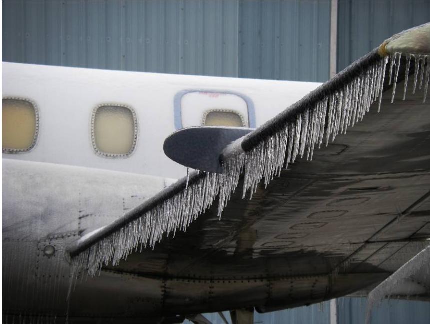
Any aircraft not parked in a hangar quickly became inoperable due to ice accumulation as a result of the December 6 storm. Above: this Fairchild Metro cargo aircraft acquired a spectacular coating of ice and icicles on its wings. Top Right: this Boeing 737-200 was similarly affected. Middle Right: some aircraft, such as this Civil Air Patrol Gippsland Aeronautics GA-8 AirVan accumulated enough ice on their tail surfaces to lift the nosewheel off the pavement. Right: a Cessna 172RG rests on its tail. Below Left: the Runway 15 Localizer antenna grew some ice whiskers. Bottom Right: all of the airport's gates iced up, requiring attention from Airport Maintenance to render them operational again. Shown here is a pedestrian gate giving access to Taxilane Sierra.
