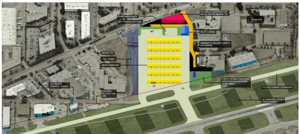
(Top) Conceptual illustration of a T-hangar development on the west side of the airport, north of the toll tunnel, with amenities including self-service fuel and a public park with an aircraft viewing area. (Bottom) Conceptual illustration of a west side development for light aircraft as viewed from the adjacent park space.
