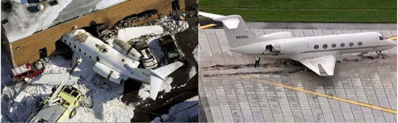
Left: runway overrun, February 2, 2005, prior to EMAS installation (13 injured). Right: October 1, 2010 overrun safely stopped by EMAS.
